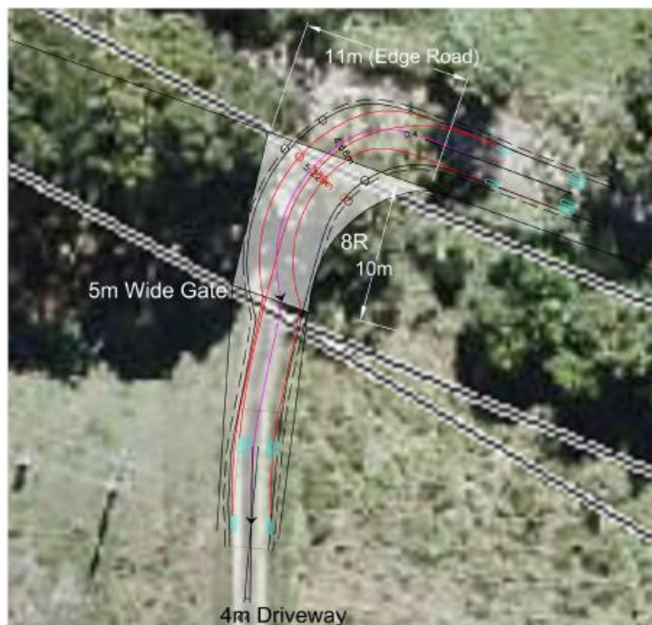
Figure 3.3 Turning Template Assessment of Works Required
