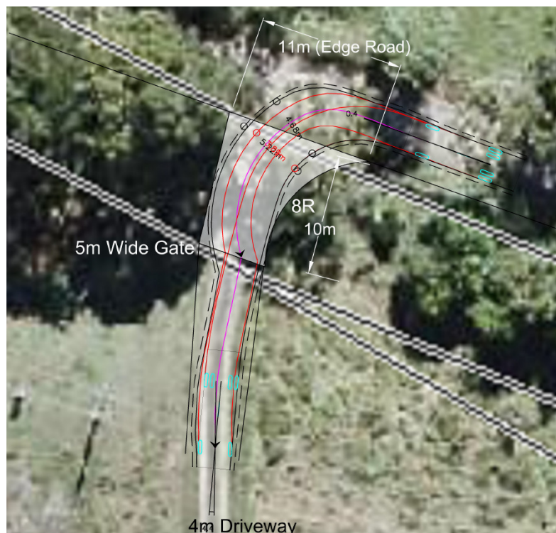
Figure 3.3 Turning Template Assessment of Works Required
