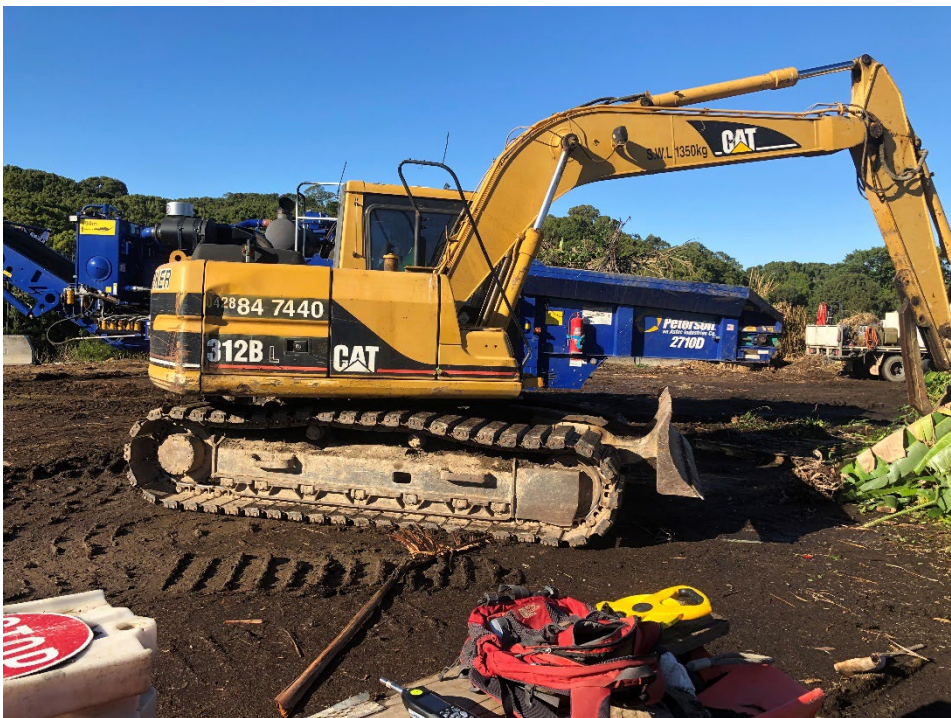
Photo B Excavator feeding Mulcher
