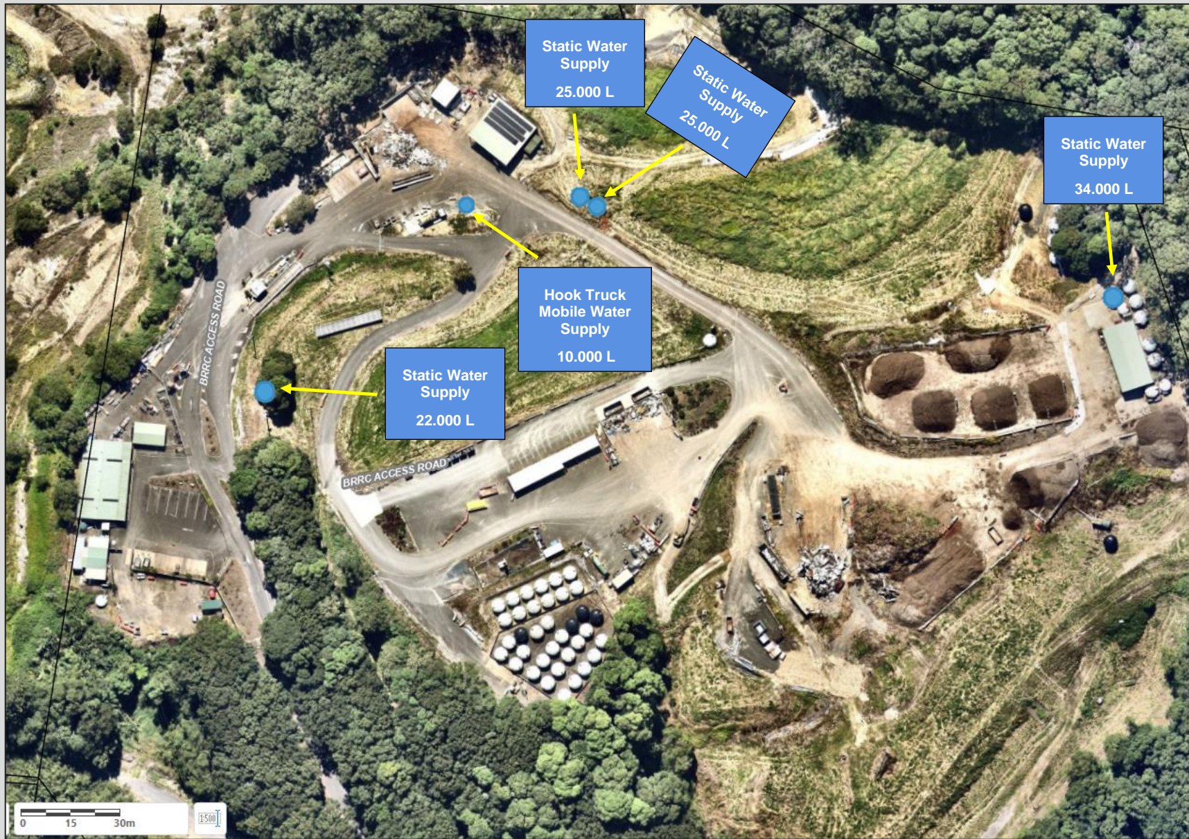
Figure 7. Firefighting static and mobile water supply.
